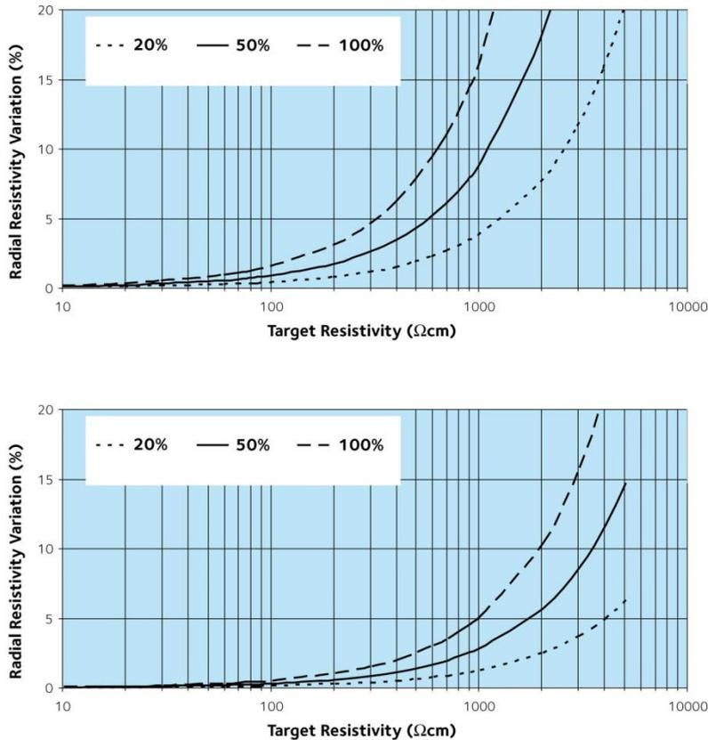
**Figure 3.** a) Radial resistivity variation of undoped silicon with average resistivity of 5000  $\Omega\text{cm}$ ,
