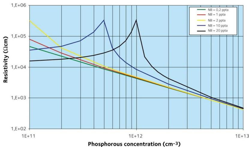
**Figure 1.** Estimated resistivities in near intrinsic silicon at 300 K versus phosphorous concentration for various background levels of boron.  $\mu_e$  and  $\mu_p$  are arbitrarily fixed at  $1500 \text{ cm}^2/\text{Vs}$  and  $450 \text{ cm}^2/\text{Vs}$ .
