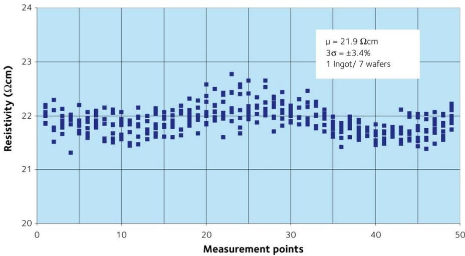
**Figure 6.** Radial resistivity variation plot for (100) p-type PFZ wafers
