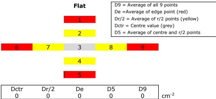
**Figure 2.** Delineation of D-defects (Flow Pattern Defect void density) by prolonged Secco etching.
