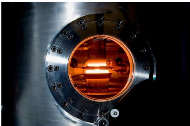
**Figure 1.** Picture of the Float Zone process. The upper part is the polysilicon rod and the lower part below the RF coil is the solidifying monocrystalline silicon rod
