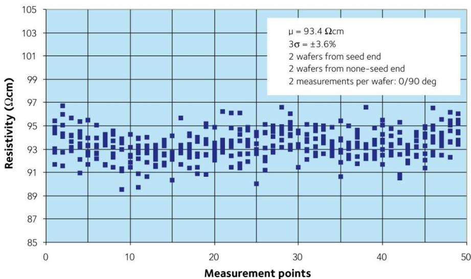
Figure 5. Resistivity tolerance plot for high resistivity (100) p-type PFZ wafers
