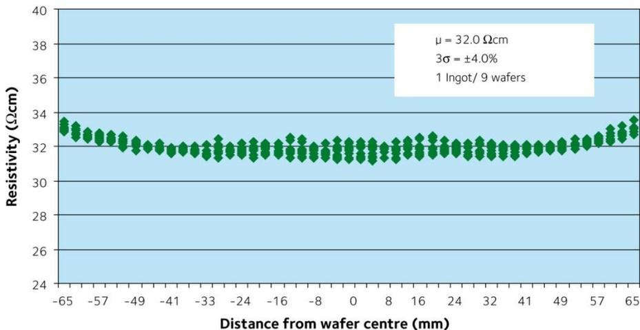
Figure 4. Radial resistivity variation plot for (100) n-type PFZ wafers
